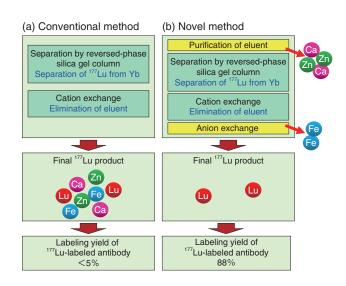
Fig.5-30 Separation of <sup>177</sup>Lu from neutron-irradiated Yb
