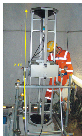
Fig.8-14 Photograph of the experimental-muon telescope
