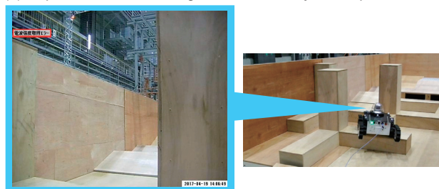
(b) Reproduction of blind region in the view by developed test field
