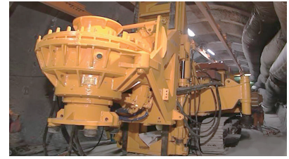
Fig.8-14 Drilling machine for a large-diameter pit
