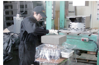
Fig.8-15 Production of a backfilling material block
