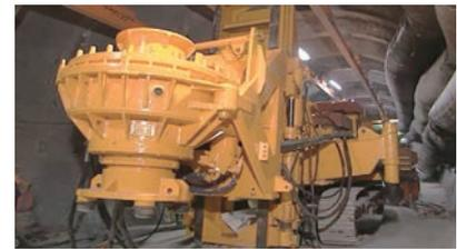
**Fig.8-14 Drilling machine for a large-diameter pit**
