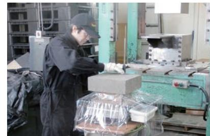
**Fig.8-15 Production of a backfilling material block**
