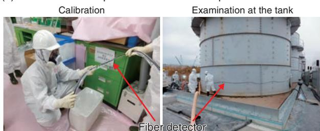
**Fig.1-24 Image of the developed fiber detector for use in monitoring contaminated-water leakage**
