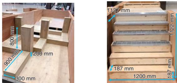
(c) Checkered iron slope test field (d) Grating floor test field
