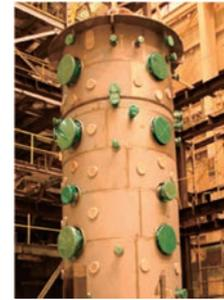
Large-scale containment vessel test facility (CIGMA)
