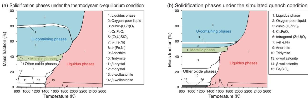
**Fig.1-8 Thermodynamically estimated solidification phases of mixed molten-core-concrete material**
