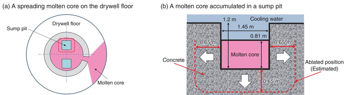
**Fig.1-7 Image of a spreading molten core on the drywell floor of a containment vessel**
