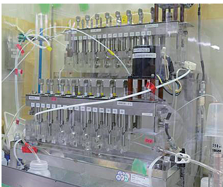
Fig.4-4 Mixer-settler extractors in a fume hood The units comprise 8-stage extraction, 8-stage scrub, and 16-stage strip sections.
