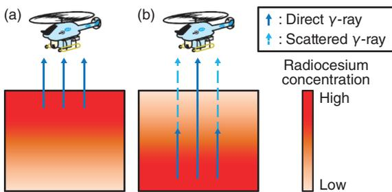
**Fig.1-23 Aerial radiation monitoring using an unmanned helicopter**
