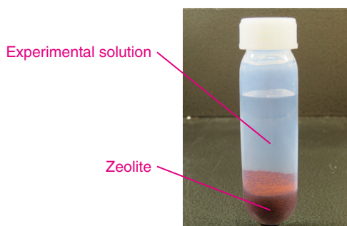
Fig.1-16 A test tube used in the sorption experiment of U and Np
