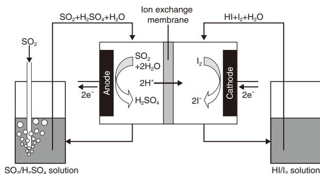
**Fig.6-15 Schematic of Bunsen reaction using ion-exchange membrane**
