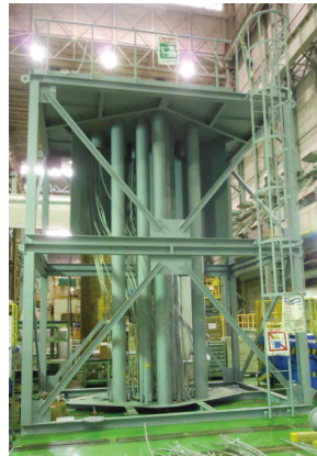
Fig.7-3 Mock-up experiment Based on the 3D-CAD study, a one-third partial full-scale mock-up was created.
