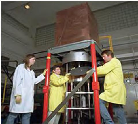
**Fig.4-15 Critical Assembly 'COMET', in the United States National Criticality Experiments Research Center (NCERC)**
