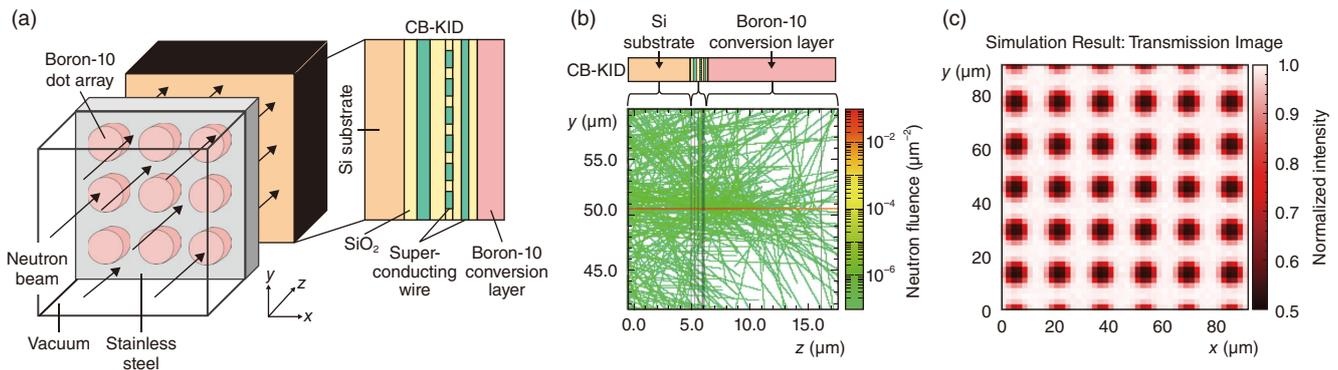
**Fig.9-4 (a) Model of the CB-KID superconducting neutron microscope, (b) PHITS simulation of radiation tracks inside the CB-KID, and (c) simulated neutron transmission image from the CB-KID**
