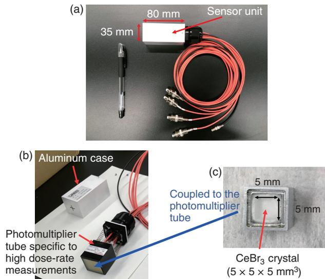
**Fig.1-4  $\gamma$ -ray spectrometry system specifically for high dose-rate measurements**
