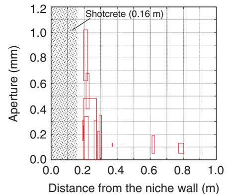
**Fig.8-19 Relationship between the fracture aperture and distance from the niche wall**
