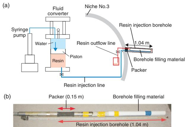
**Fig.8-17 (a) Experimental setup for resin injection tests and (b) photograph of the packer system used in the resin injection borehole**
