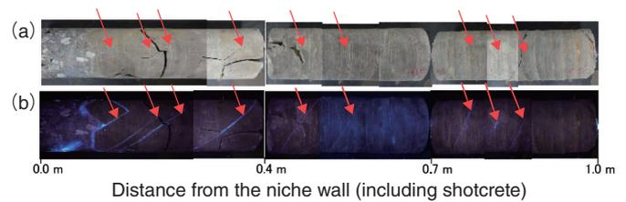
**Fig.8-18 Photographs of the injection borehole taken under (a) natural and (b) UV light**
