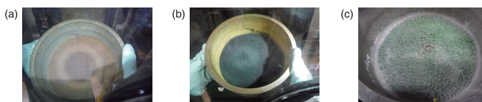
Fig.8-8 Change in the appearance of nuclear fuel material containing organic compounds subjected to heat treatment: (a) before heat treatment, (b) after heat treatment (200 °C), and (c) after heat treatment (700 °C)
