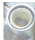
Fig.3 NpPd 3 sample obtained by the reaction of neptunium nitride with Pd
