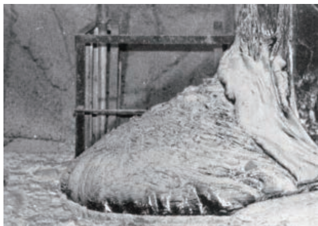
Fig.1 “Elephant foot” observed immediately after the accident*1 Fuel debris shaped like an elephant's foot was formed during the Chernobyl NPP accident that occurred in 1986. It was very hard, glassy, black, lava-like materials with very high radioactivity and a large amount of concrete components.
