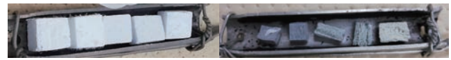
Fig.2 Appearance of thermal insulation before and after the chemisorption test with Cs vapor
